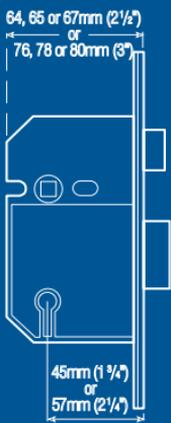
Mortice locks are sized by the depth of the lock case and the rectangular hole – the “mortice” – into which the lock fits.
