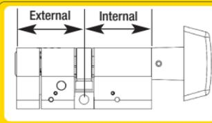
For thumb turn cylinders, the first size on the product code indicates the side the thumb turn is on. The Anti-Snap protection is on the external side of the cylinder.
