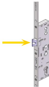
**Push the latch into the gearbox into its hold-back position to activate the snib feature.**
