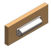
4. Secure in place from the internal side using x4 M4 fixing screws provided. To avoid distortion and over-compression of the gasket please ensure the screws are not over tightened.
