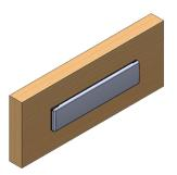
2. Position the external letterplate assembly into the aperture
