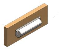
5. Push 4 screw cover caps into place and remove the protective film
