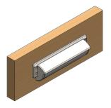
3. Repeat this step positioning the internal letterplate assembly into the aperture.
