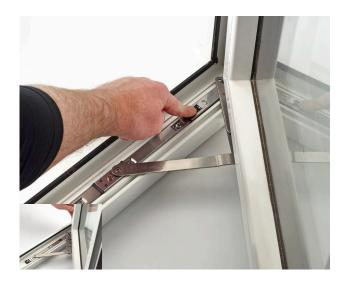
3. To activate the "Easy Clean" mode push both black slide buttons (top and bottom) towards the corner and slide the Sash away.
