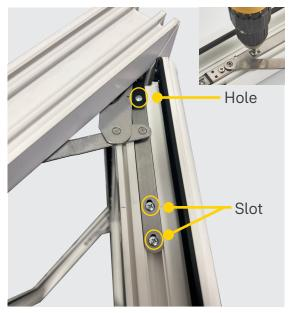
2. Insert countersunk screws into the 2 slots and then make adjustments to Sash position if required. Then insert screw into the screw hole.
