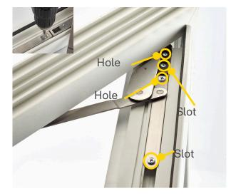
2. Insert countersunk screws into the 2 slots and then make adjustments to Sash position if required. Then insert screw into the 2 holes.
