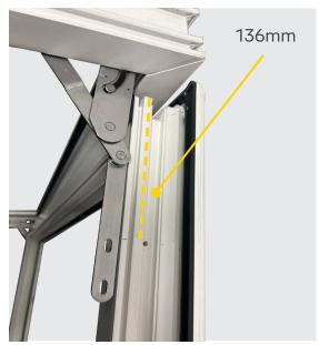
136mm is the distance from the edge of the Sash rebate to the middle of the first slot on the Sash.
