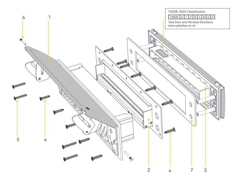
**N.B.** Fasteners used to secure the product must be suitable for the substrate material. Use of exterior silicone sealant is required (not supplied).
