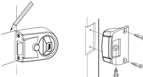
Close the door and using the lock case as a guide mark the position of the remaining component – the 'staple' – on the door frame. Chisel out a recess in the door frame to hold the staple flush with the frame and fix it with the screws provided.
