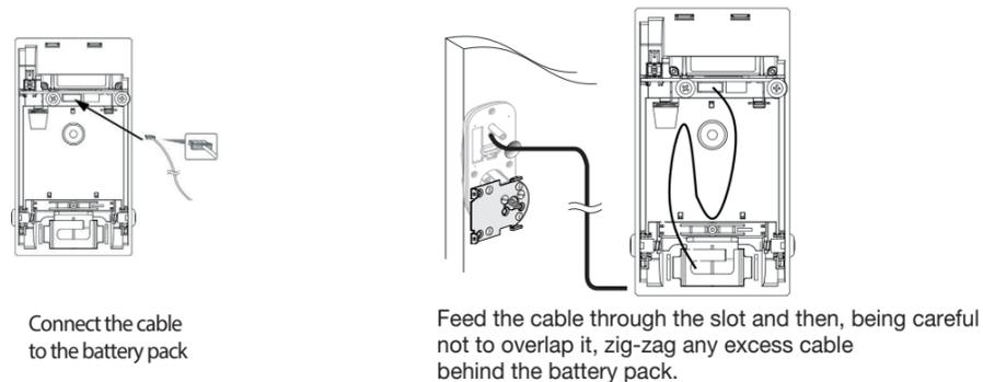
Connect the cable to the battery pack
