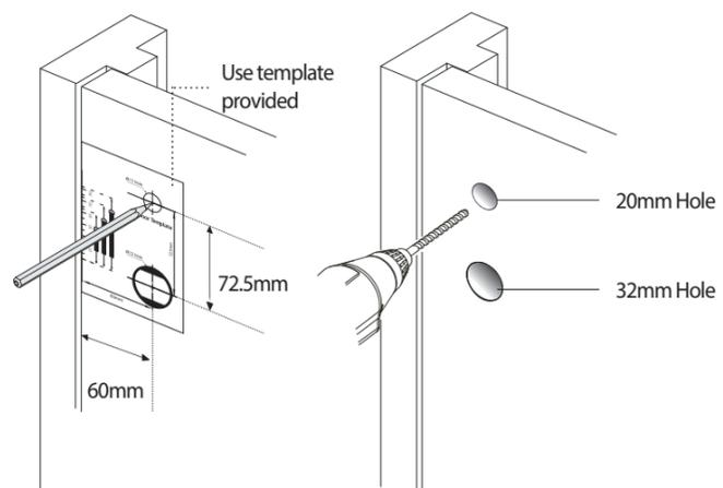
At the height you want your lock, use a pencil to mark a spot exactly 60mm from the edge of the door. At that spot, drill a 32mm diameter hole through the door.
