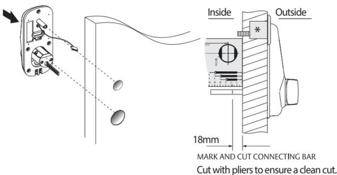
Place the electronic keypad in the hole on the outside of the door.
