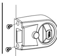
Repeat step 7 to position the lock case flush with the edge of the door. Secure the lock case to the mounting plate with the two small screws provided.
